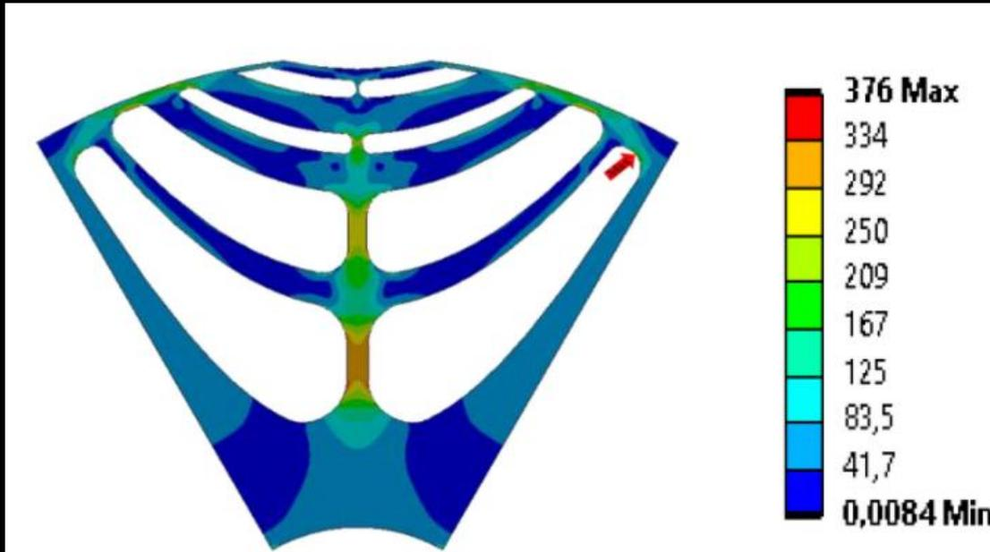
Initial Optimised design rotor lamination
