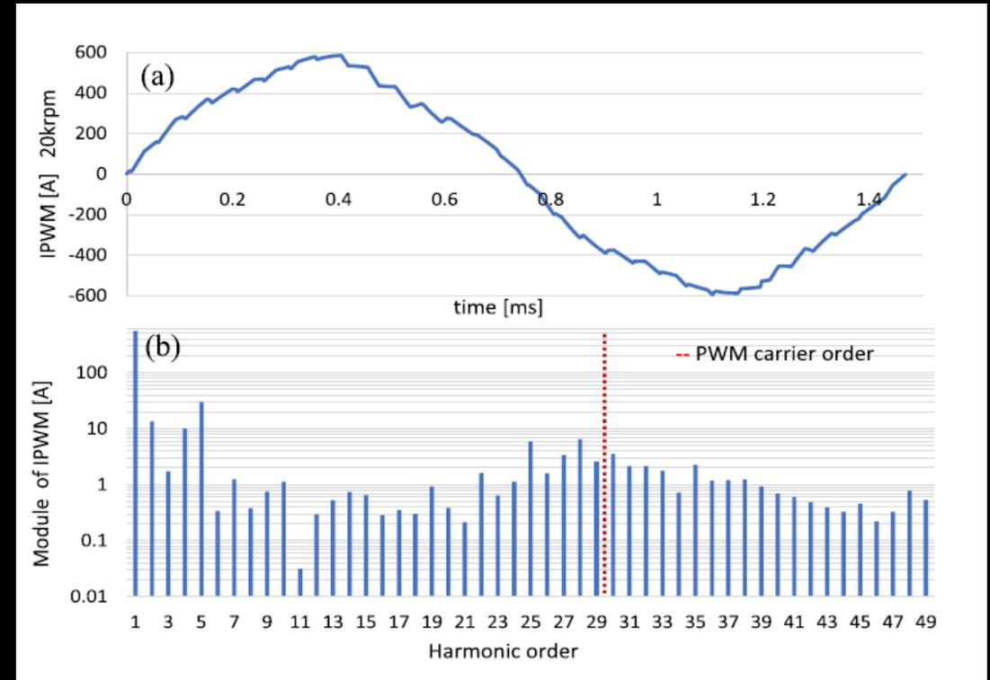
Current waveform @ 96 Nm, 20 krpm, 680.3 Hz fundamental frequency, 20 kHz PWM carrier
