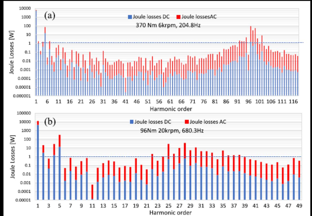
Ohmic Losses (a) 6 krpm, 204.8 Hz fundamental frequency, 20 kHz PWM carrier; (b) 20 krpm, 680.3 Hz fundamental frequency, 20 kHz PWM carrier
