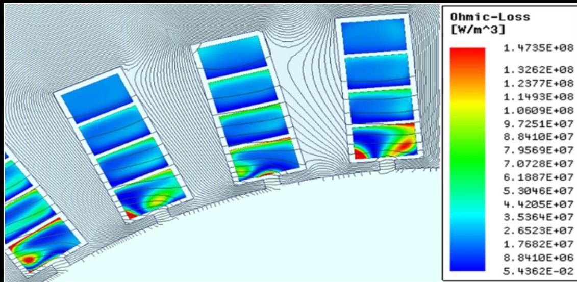
Ohmic Losses distribution @ 96 Nm, 20 krpm, 680.3 Hz fundamental frequency, 20 kHz PWM carrier
