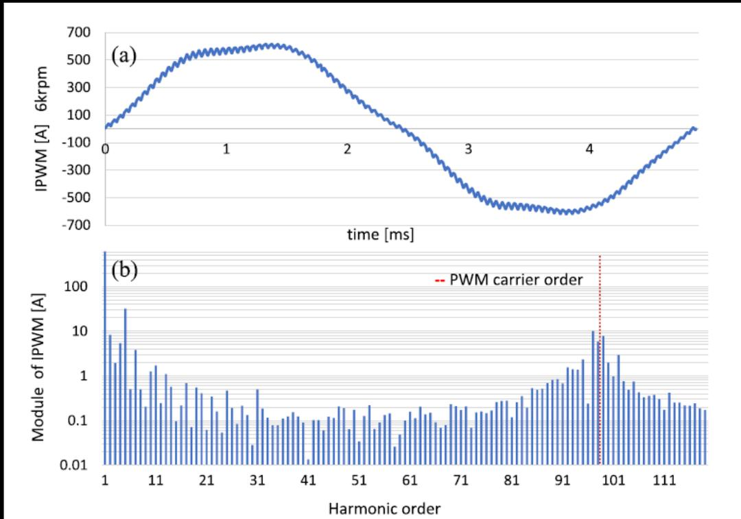
Current waveform @ 370 Nm, 6 krpm, 204.8 Hz fundamental frequency, 20 kHz PWM carrier
